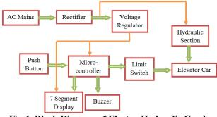
Fig 4: Block Diagram of Electro-Hydraulic Goods **Elevator**
